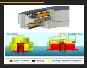
LINTECH Slewing bearing, also known as turntable bearing, is a crucial component in a Single Point Mooring (SPM) system which functions as: allow rotation, support heavy loads, provide stability, facilitate smooth movement, absorb external forces.
