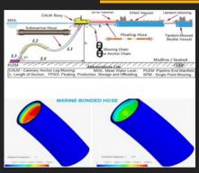
LINTECH SPM mooring analysis is a process that involves calculating the forces acting on a Single Point Mooring (SPM) system, and analyzing the tension of each mooring line.
